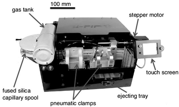
**Fig. 5 Photograph of an instrument for controlled, automated, continuous production of fused silica micropipettes**
