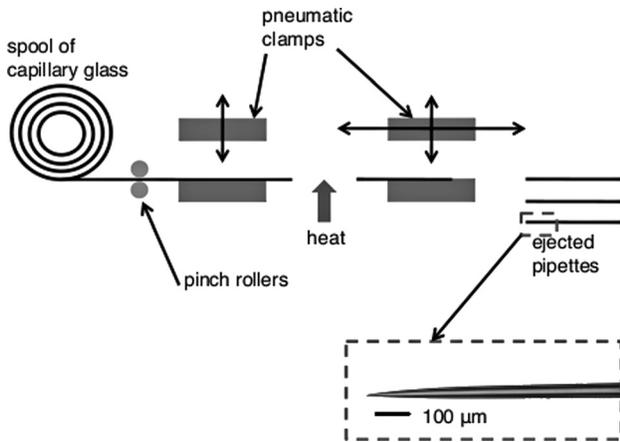
**Fig. 2** The basic operation of a fully automated micropipette puller. The inset shows a microscope image of a pulled micropipette manufactured using our machine.
