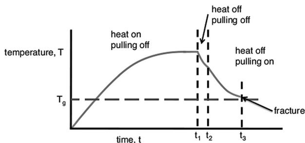
**Fig. 1 A conceptual heating and cooling model for pulling a micropipette. The amount of time it takes to cool the pipette back to the glass transition temperature determines the geometry.**
