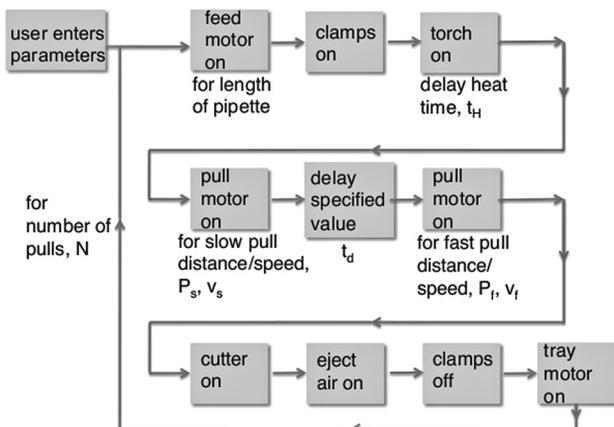
**Fig. 6 The sequence of events that the pipette pulling program runs. The user inputs the number of pipettes,  $N$ , length, heat time,  $t_H$ , slow pull speed,  $v_s$ , slow pull distance,  $P_s$ , fast pull speed,  $v_f$ , fast pull distance,  $P_f$ , and delay,  $t_d$ .**
