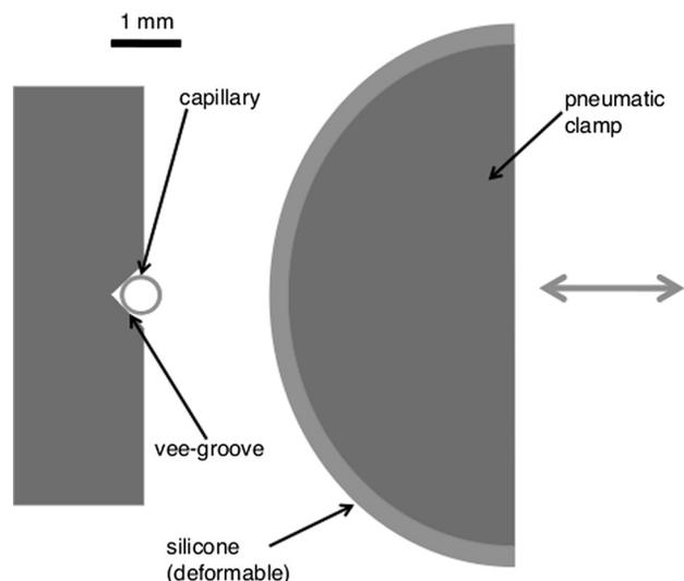
**Fig. 4** Diagram of pneumatic clamp and vee-groove used to secure both ends of the capillary for pulling
