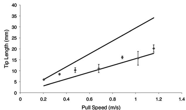
**Fig. 7 Relationship between pull speed and micropipette tip length, with standard deviation.  $N=10$ ,  $t_H=14$  s,  $v_s=0.27$  m/s,  $P_s=2.54$  mm,  $P_f=22.9$  mm,  $t_d=70$  ms, and a varied  $v_f$  as indicated. The solid lines indicate the upper and lower bounds achieved using our thermal model and Eq. (4).**
