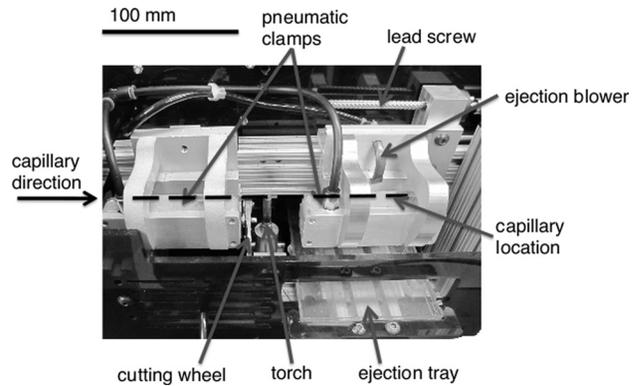
**Fig. 3** Photograph of the main mechanical and thermal components of a fully automated micropipette puller
